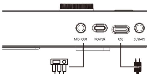
Use with external MIDI device: Use a 3.5mm TRS to MIDI DIN adapter(not included) plug into the MIDI OUT of Vboard 49, then connect to the MIDI IN of external MIDI device through a 5 pin MIDI cable, turn on the power of Vboard 49. Please see [6.4 MIDI DIN to 3.5mm TRS Adapter](#) for more details.
