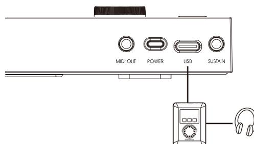
Use with **MIDIPLUS** miniEngine series sound engine: Connect Vboard 49 to the USB Host of miniEngine using the included USB cable and turn on the Vboard 49, connect your speaker or headphone to miniEngine and turn on the miniEngine.
