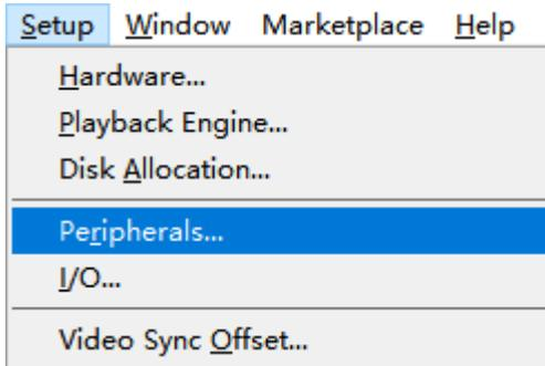
2. In the pop-up window, click on the **Machine Controllers** tab, find the **MIDI Machine Control Remote (Slave)** and click it, set the ID as 116, then close the window to finish setup.
