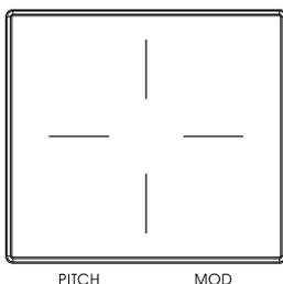
The Touch Pad allows you to control the Pitch bend and Modulation. By default, touch the left side to control Pitch bend and touch the right side to control Modulation. Hold down the SHIFT button then pressing the key labeled with "Touch Pad" to switch to XY Pad mode, when in XY Pad mode, the axis X is assigned to CC71 and axis Y is assigned to CC74.
