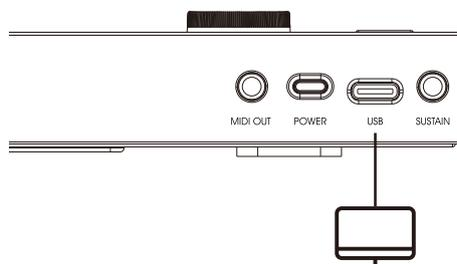
Use with computer: Connect Vboard 49 to your PC or Mac using the included USB cable and turn on the power. Vboard 49 is a class-compliant USB device, so its driver are automatically installed when connecting to a computer.
