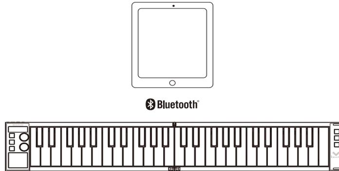
Connect to iOS device: Turn on the Vboard 49 power button and switch on bluetooth on the iOS device, then open the app which support Bluetooth MIDI and connect Vboard 49 in setup menu. Please refer to [5. Bluetooth MIDI Connect \(iOS\)](#) for detailed operation steps.
