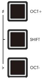
Pressing the OCT+ or OCT- button to shift the octave range of keyboard, Pressing the OCT+ and OCT- buttons simultaneously will quickly reset the octave shift.
